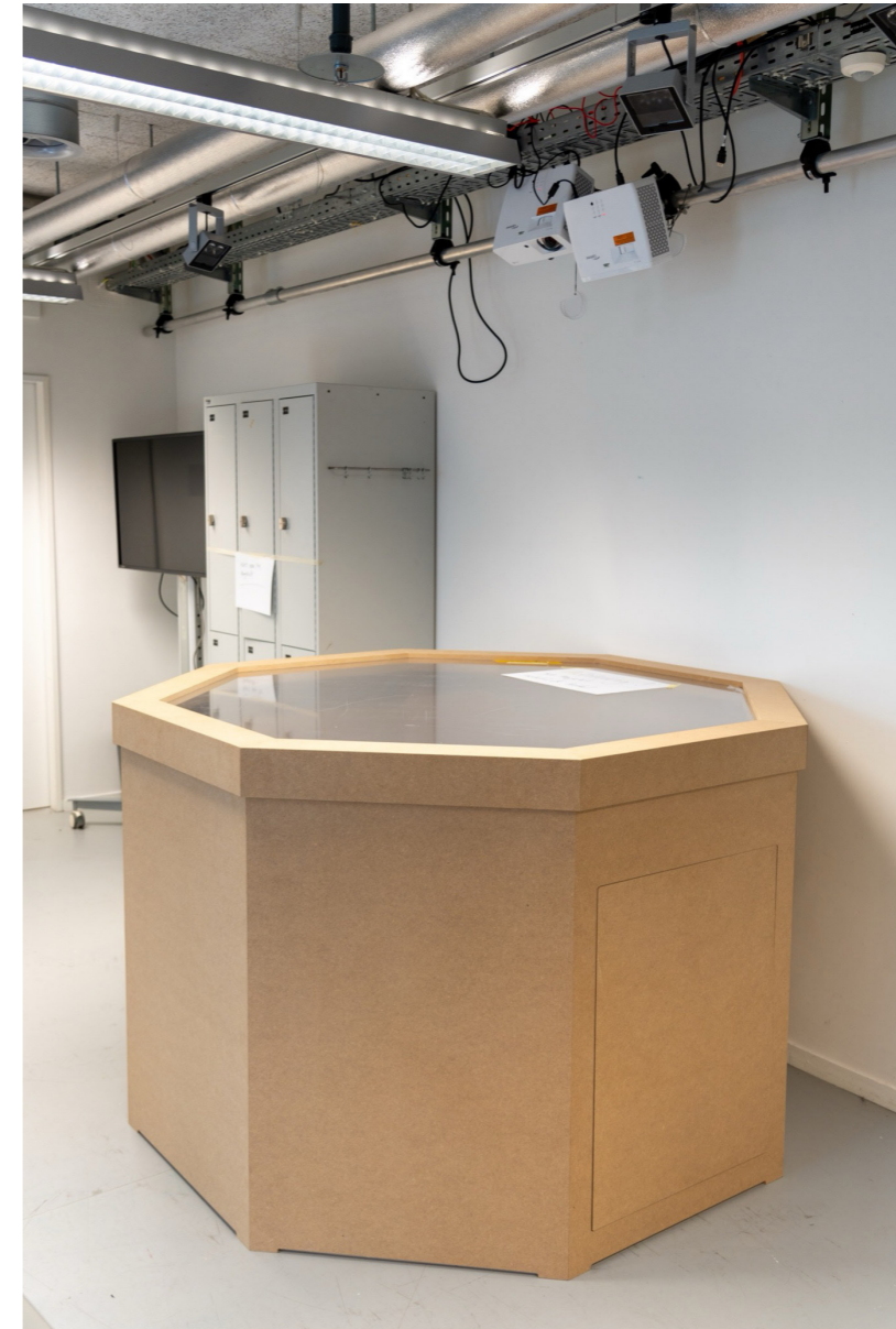
Figure 43 assembled table with MDF and plexiglass
