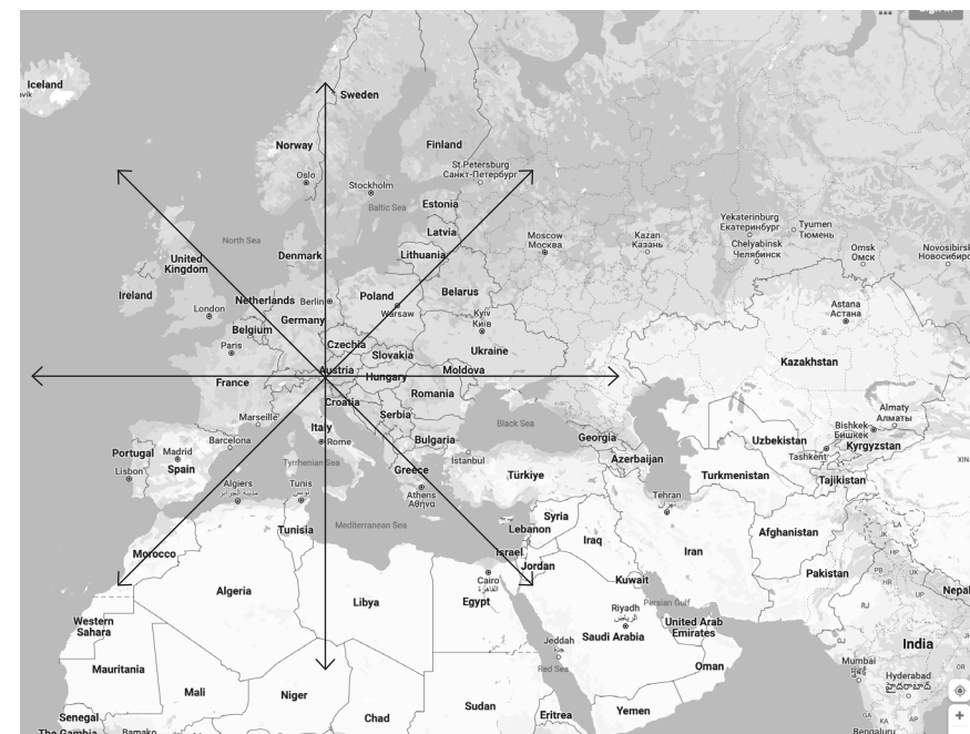
Figure 50: Size of compass sector increases along with distance
