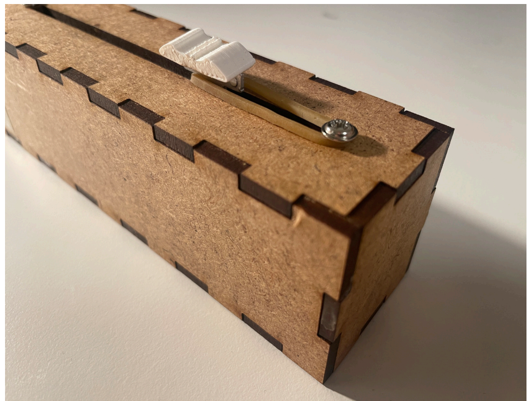
Steurer Jene, S. (2023). Fig.39: Rubberband fader enclosed in a box
