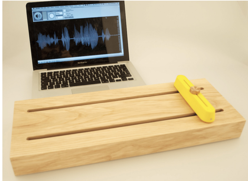
Parkinson A., Tanaka A. (2016). Fig.29: Haptic Wave a cross-modal interface for visually impaired audio producers. https://doi.org/10.1145/2858036.2858304
