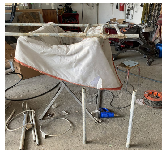
F60 After I removed the four-place headliner, my father, a body builder, welded the pieces together.
